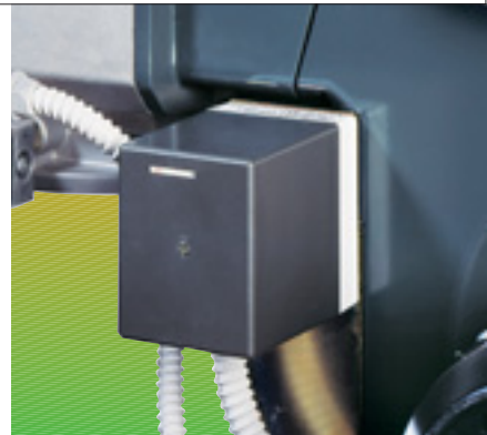
Example of the servomotor for air/gas setting
