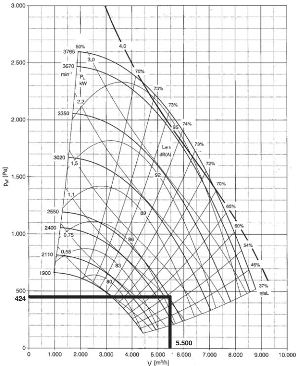
Now check the operating point on the fan graph on page 28 It shows that the fan is working within performance limits.
