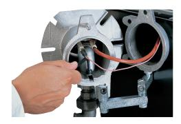
Riello 40 GS burners are fitted with an air pressure switch which, in accordance with EN 676 standards, can be adjusted by the installer using a graduated selector, on the basis of the effective working conditions.
