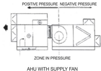
and this condition is automatically verified using the dimensioning suggested for the inlet fan.
